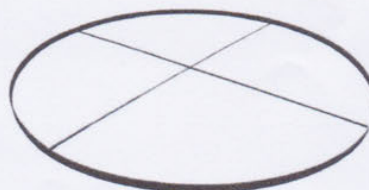
Steel shot circle intended to be set in concrete shot pad. Diameter of 2135mm.
