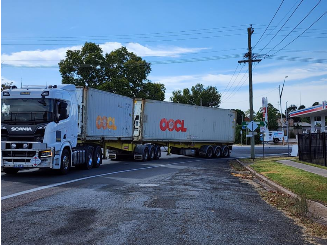
Fig 3: Intersection looking east from Audley St – B-Double turning (noting the angle of rear trailer)
