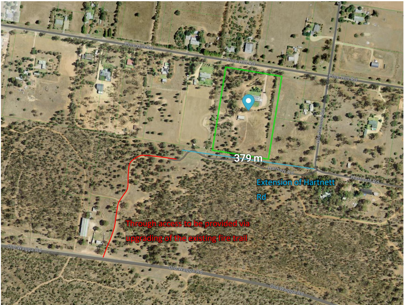
Figure 14: 2wd All weather through access to be provided for Hartnett Rd to Old Wagga Rd
