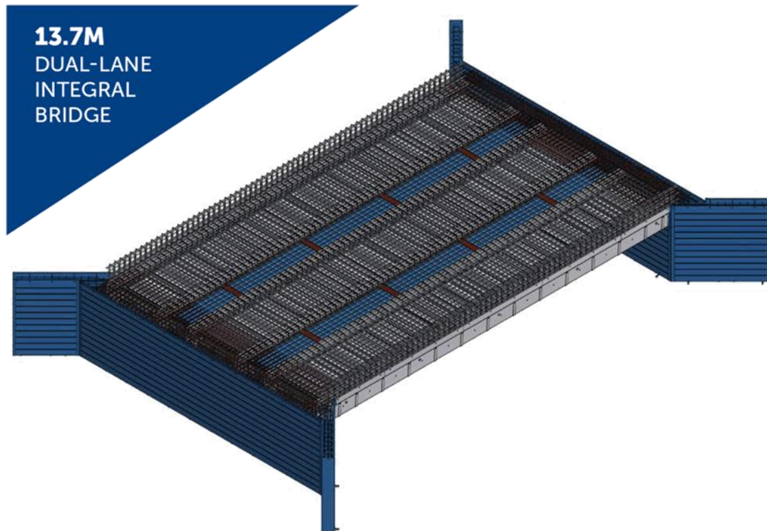
3-panel, dual-lane bridge with kerb
