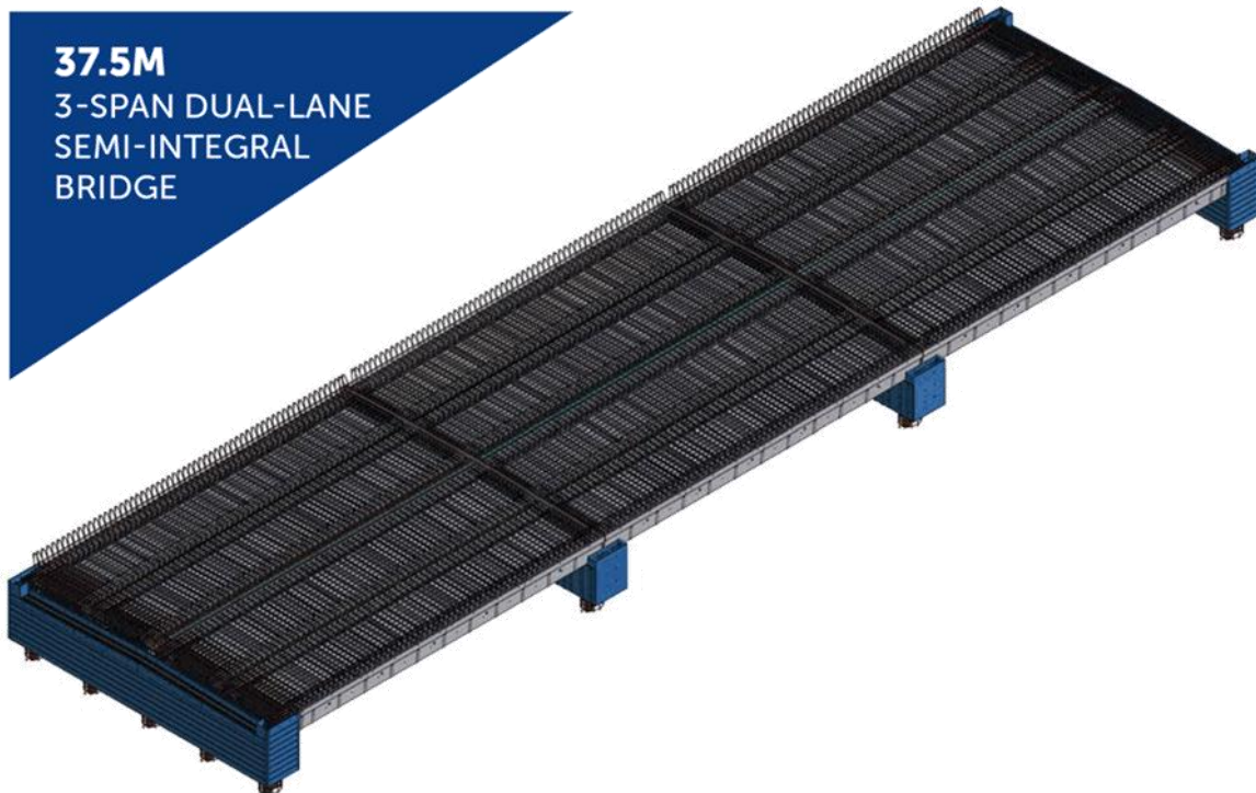
Multi-span dual-lane semi-integral bridge with concrete barrier
