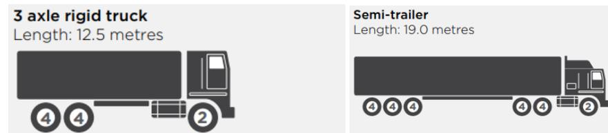
Figure 28 Heavy vehicle lengths (Source: <https://www.rms.nsw.gov.au>)
