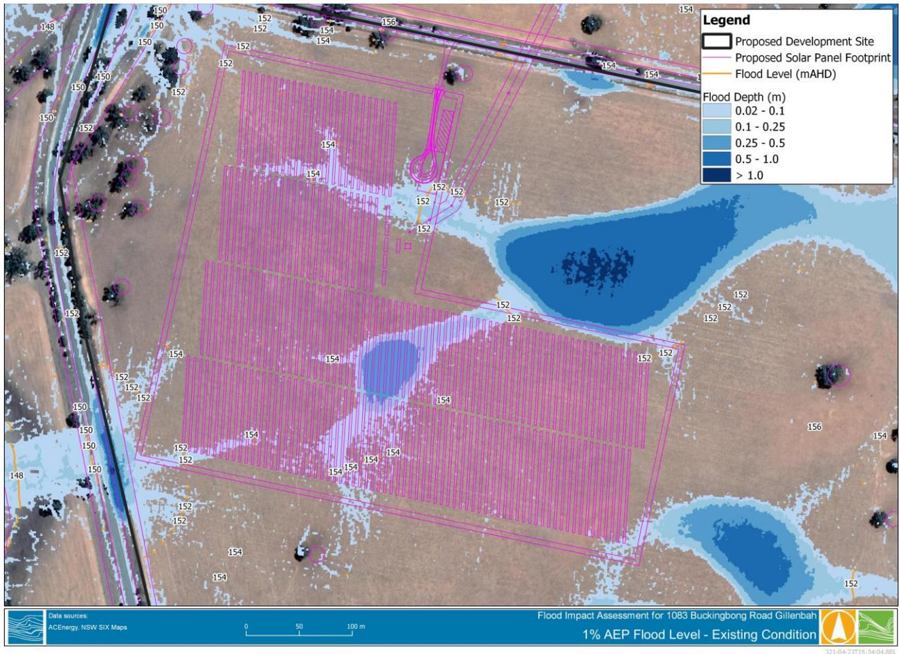
**FIGURE 7-11 1% AEP FLOOD LEVEL – EXISTING CONDITION**
