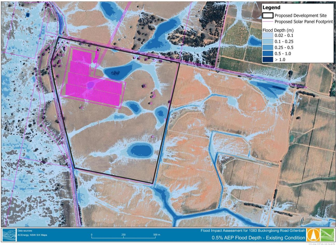
**FIGURE 7-3 0.5% AEP FLOOD DEPTH – EXISTING CONDITION**
