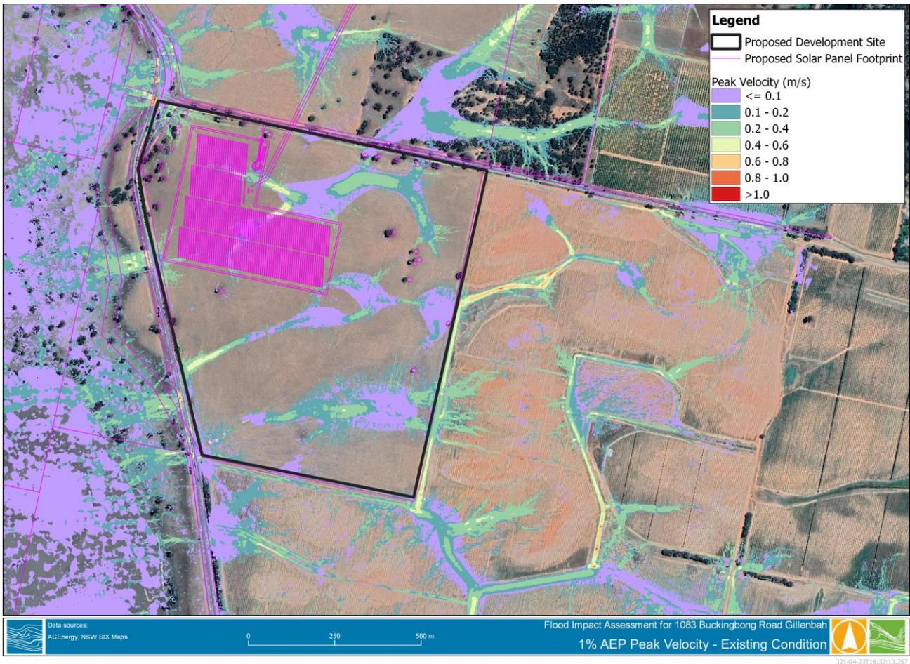
**FIGURE 2-5 1% AEP PEAK VELOCITY**
