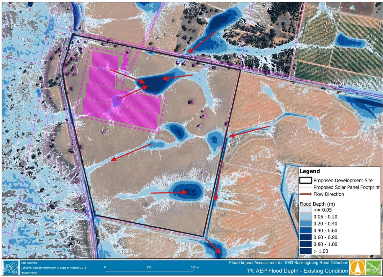
**FIGURE 3-1 1% AEP FLOOD DEPTH SHOWING PRIMARY FLOW DIRECTION**
