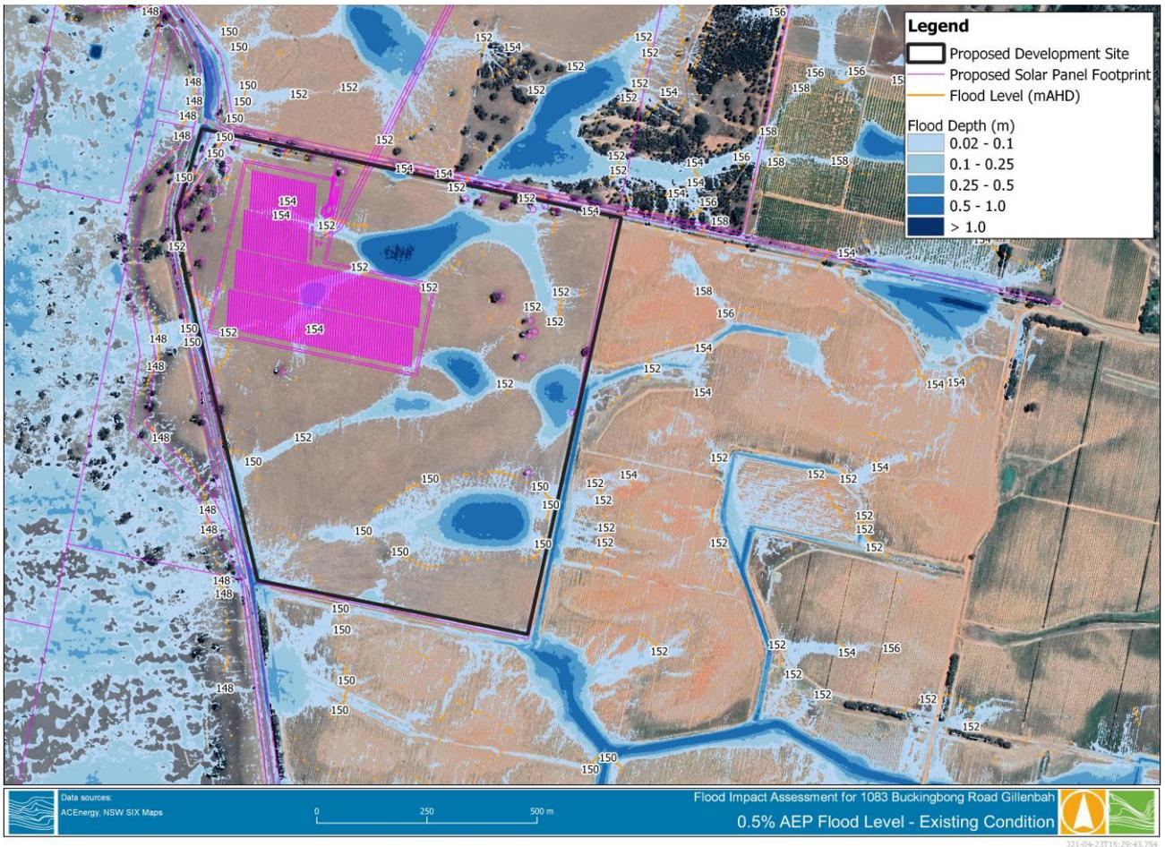
**FIGURE 7-12 0.5% AEP FLOOD LEVEL – EXISTING CONDITION**
