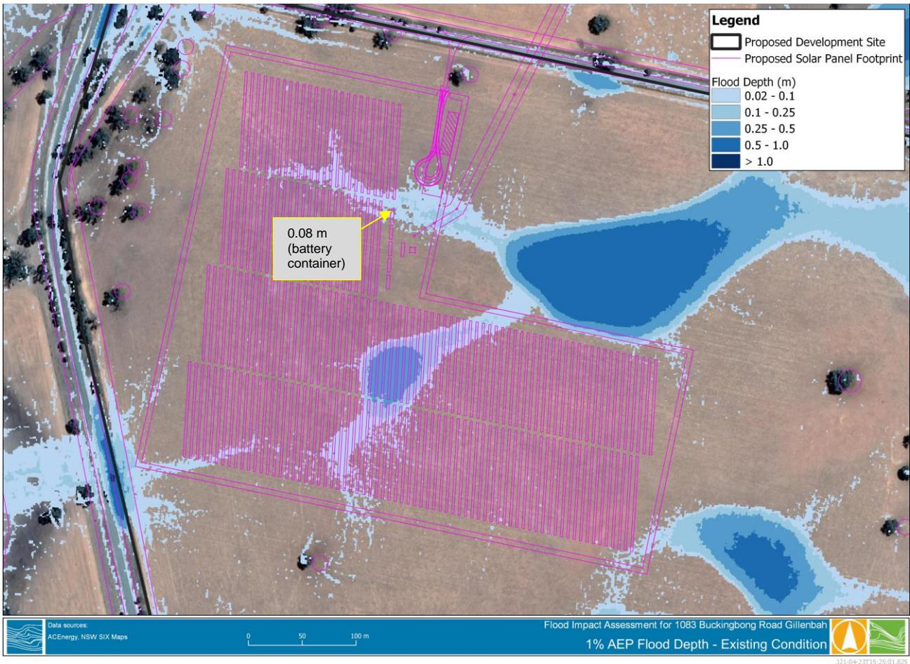
**FIGURE 2-8 1% AEP FLOOD DEPTH - AT SITE LOCATION**
