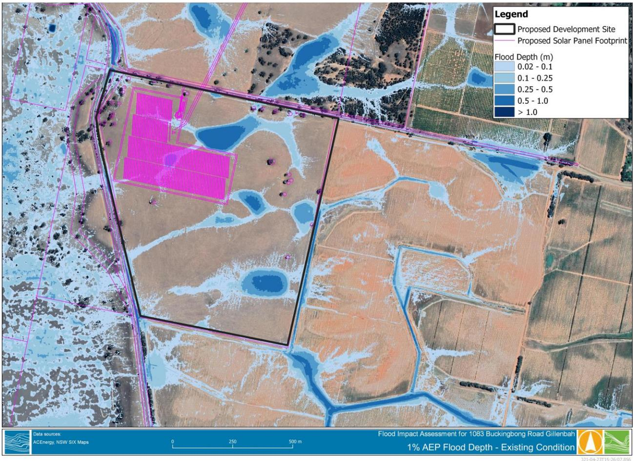
**FIGURE 7-2 1% AEP FLOOD DEPTH – EXISTING CONDITION**
