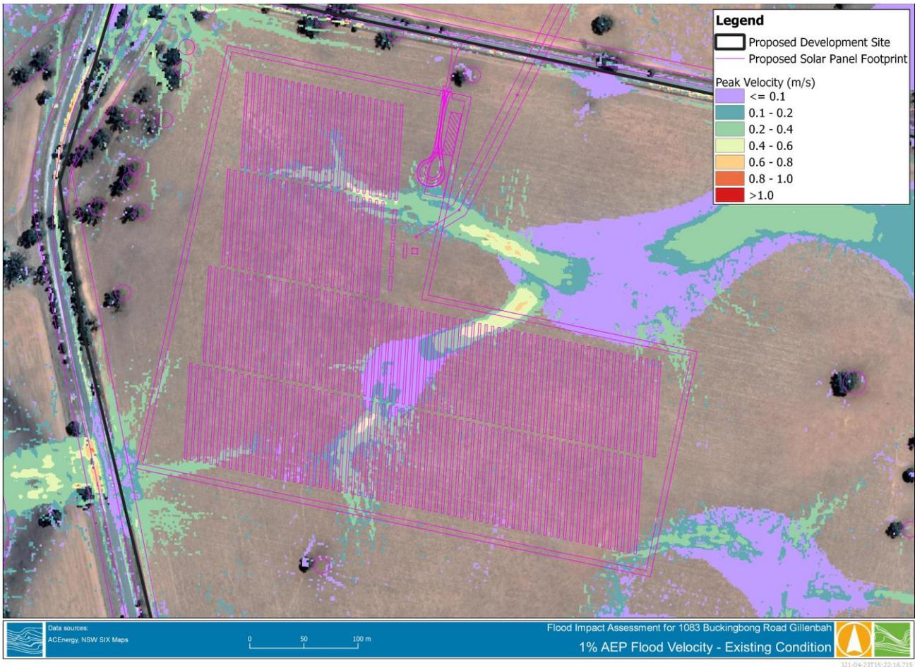
**FIGURE 2-9 1% AEP PEAK VELOCITY - AT SITE LOCATION**
