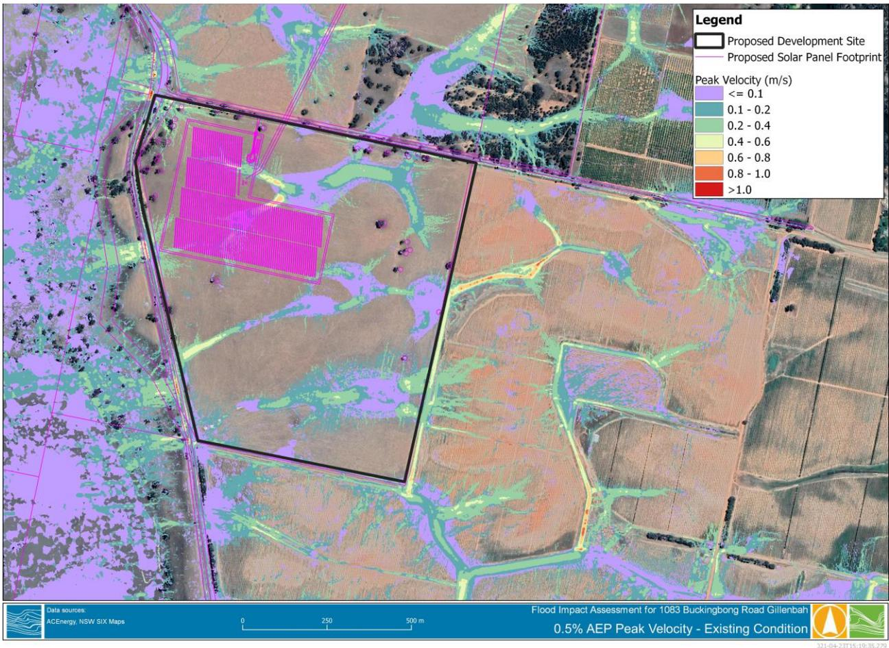
**FIGURE 7-6 0.5% AEP PEAK VELOCITY – EXISTING CONDITION**
