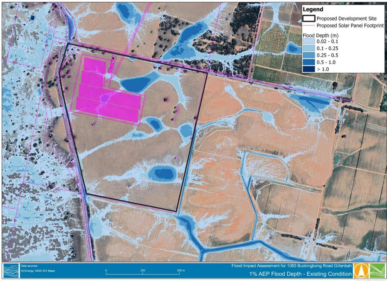
**FIGURE 2-4 1% AEP FLOOD DEPTH**
