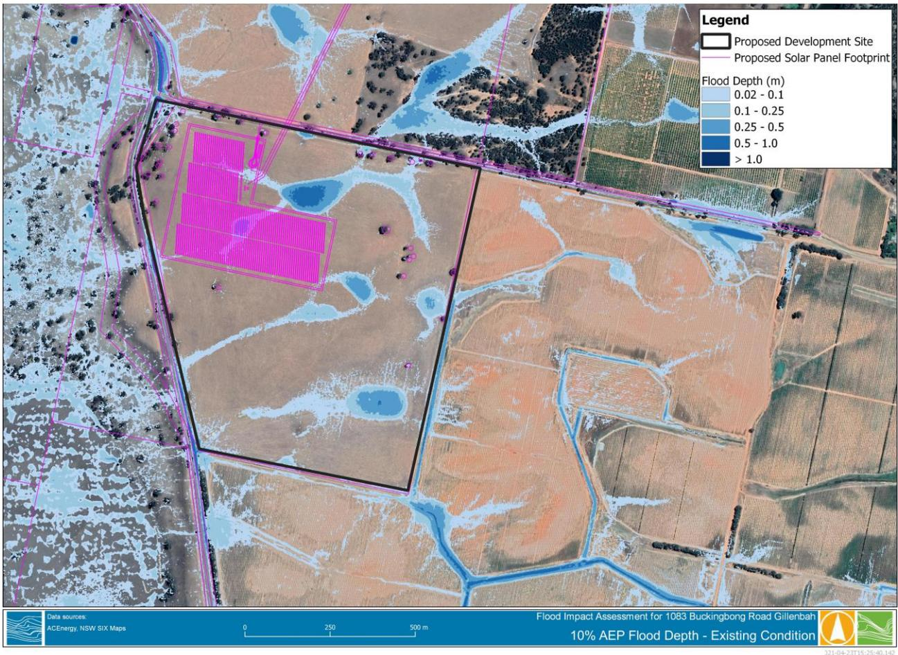
**FIGURE 7-1 10% AEP FLOOD DEPTH – EXISTING CONDITION**
