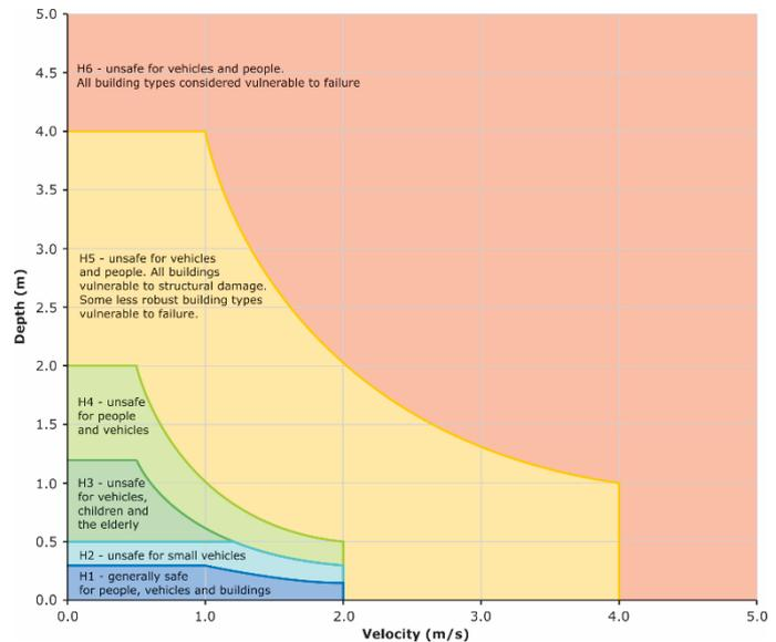
**FIGURE 2-3 COMBINED FLOOD HAZARD CURVES**
