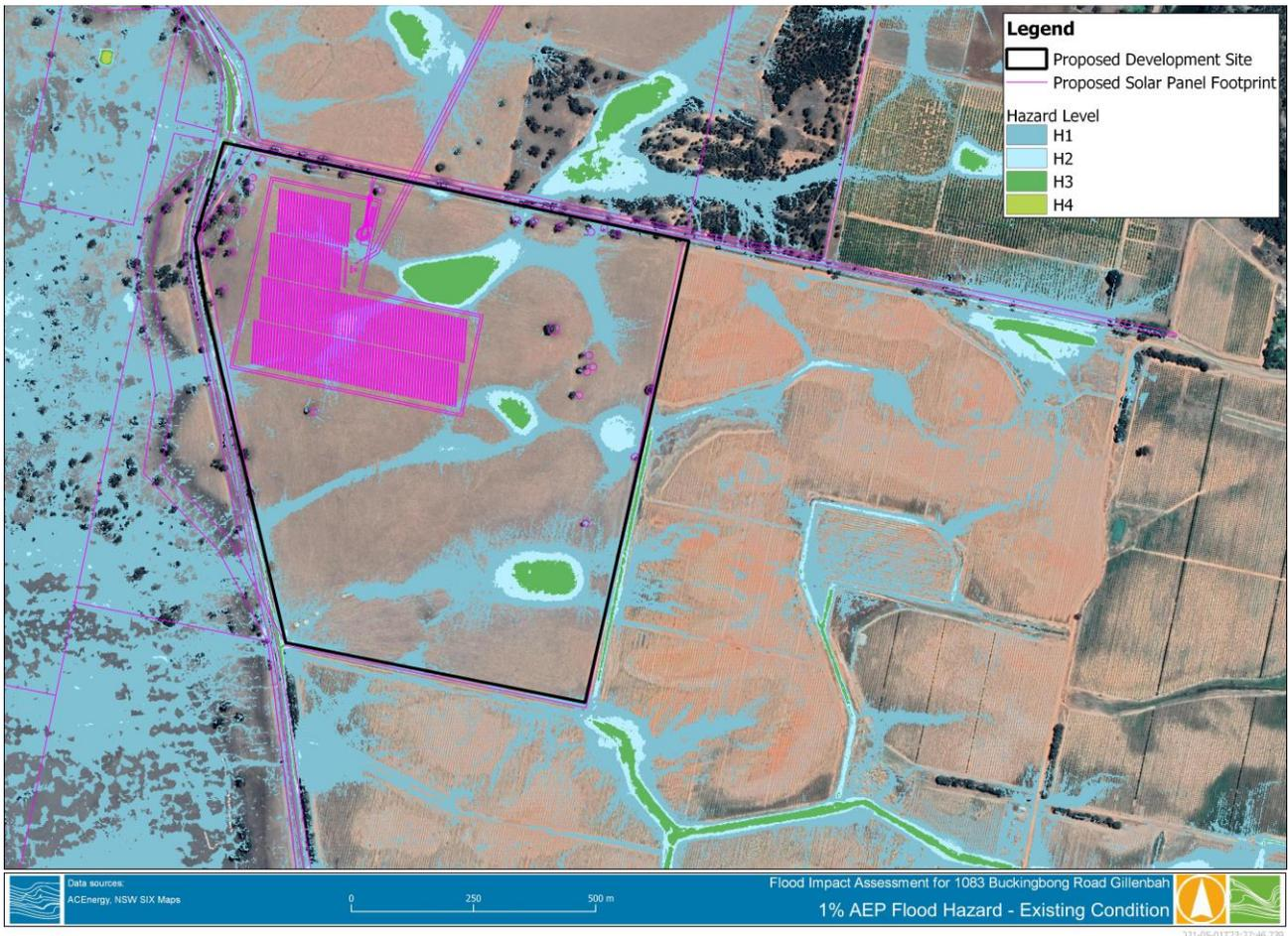
**FIGURE 2-6 1% AEP FLOOD HAZARD**
