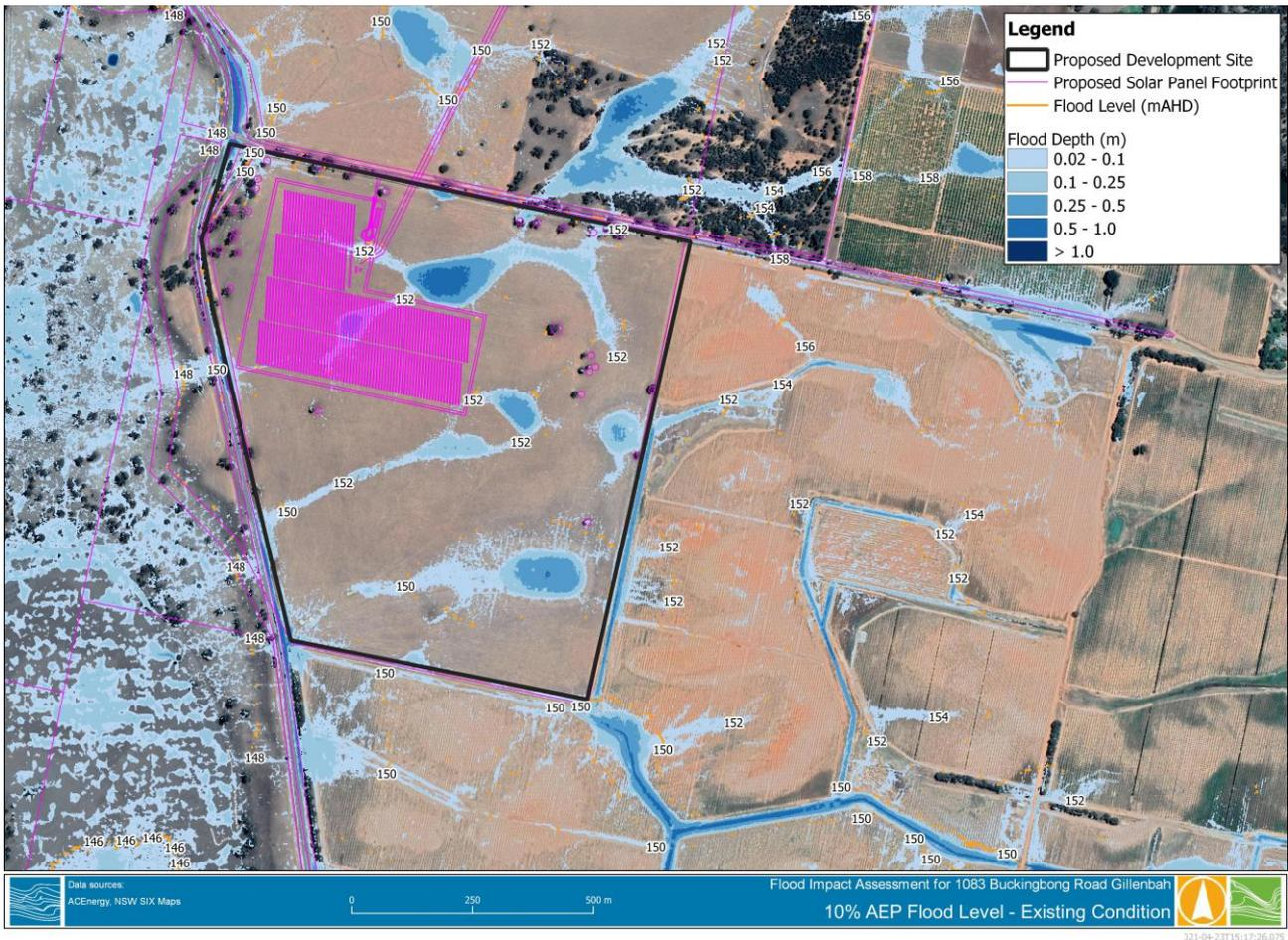
**FIGURE 7-10 10% AEP FLOOD LEVEL – EXISTING CONDITION**
