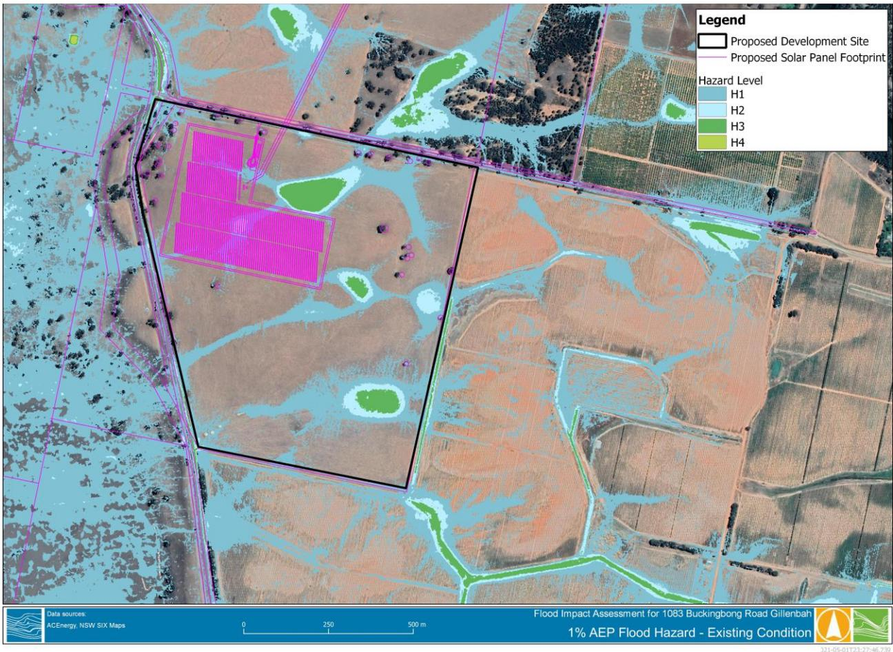
**FIGURE 7-8 1% AEP PEAK FLOOD HAZARD – EXISTING CONDITION**
