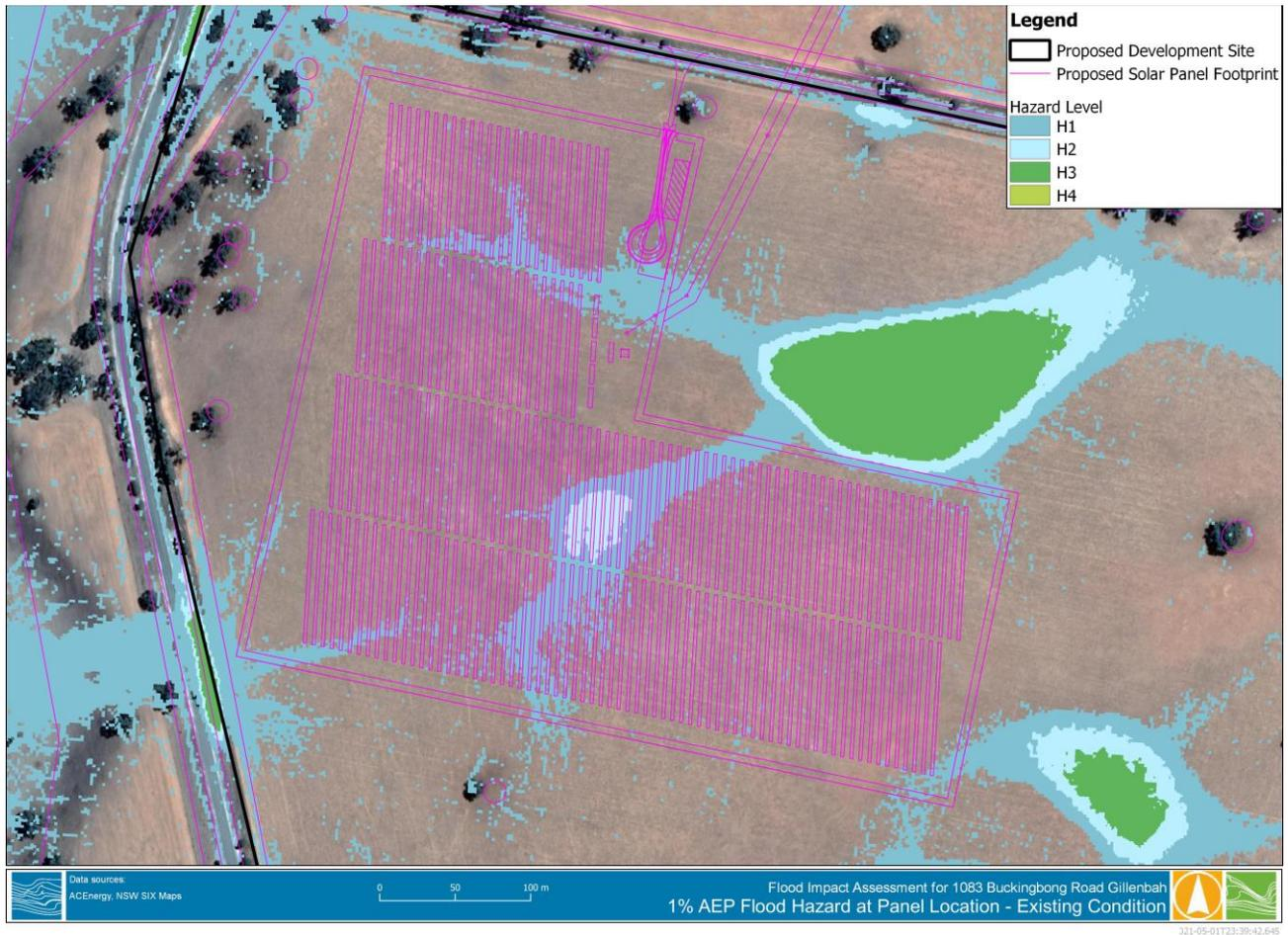
**FIGURE 2-10 1% AEP PEAK HAZARD – AT SITE LOCATION**
