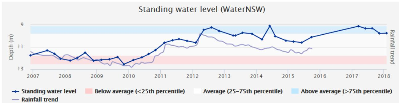
FIGURE 4-3 GROUNDWATER HYDROGRAPH FOR WATER NSW MONITORING WELL GW403567.1.1
