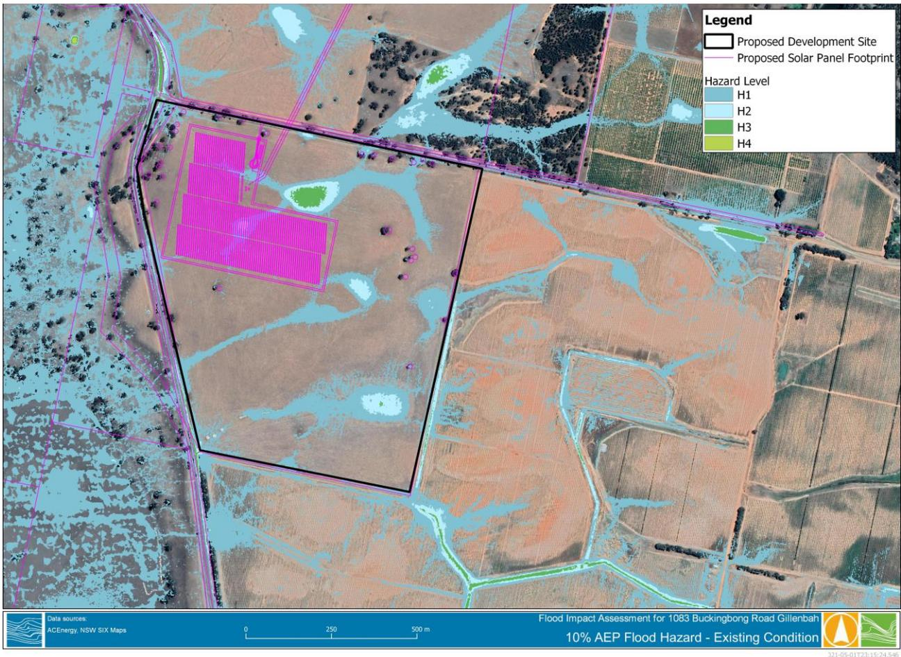
**FIGURE 7-7 10% AEP PEAK FLOOD HAZARD – EXISTING CONDITION**
