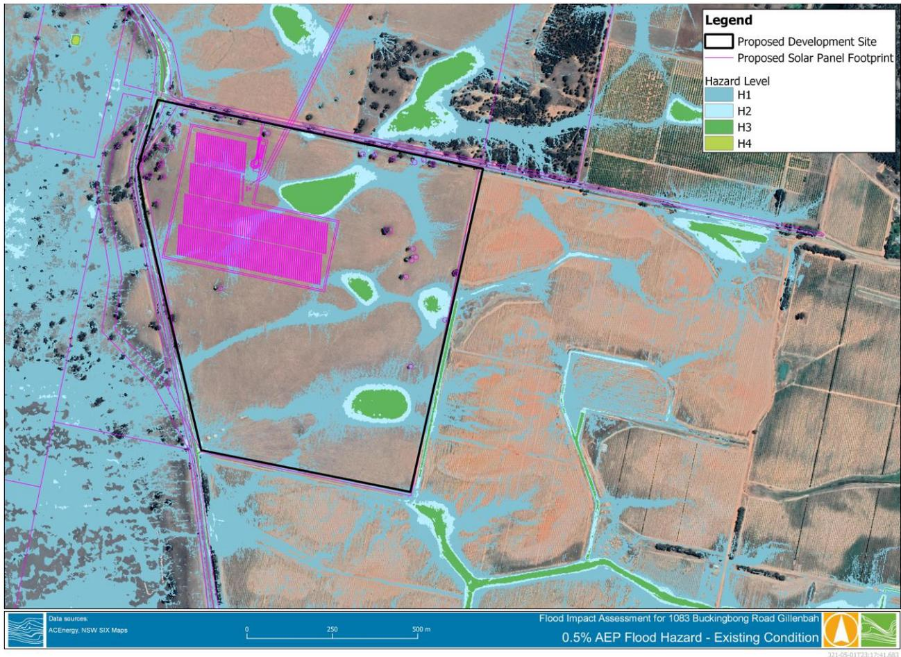
**FIGURE 7-9 0.5% AEP PEAK FLOOD HAZARD – EXISTING CONDITION**
