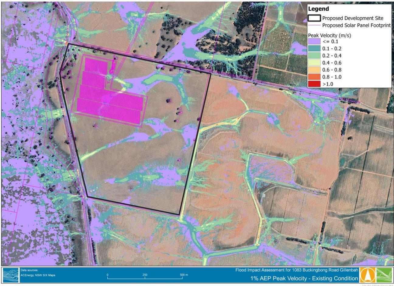
**FIGURE 7-5 1% AEP PEAK VELOCITY – EXISTING CONDITION**
