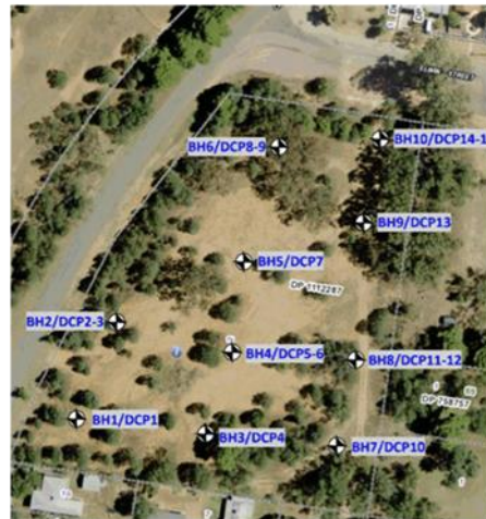
FIG 4: Borehole locations on site
