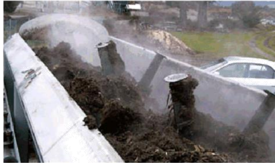
Central rotating shaft mixes and aerates
