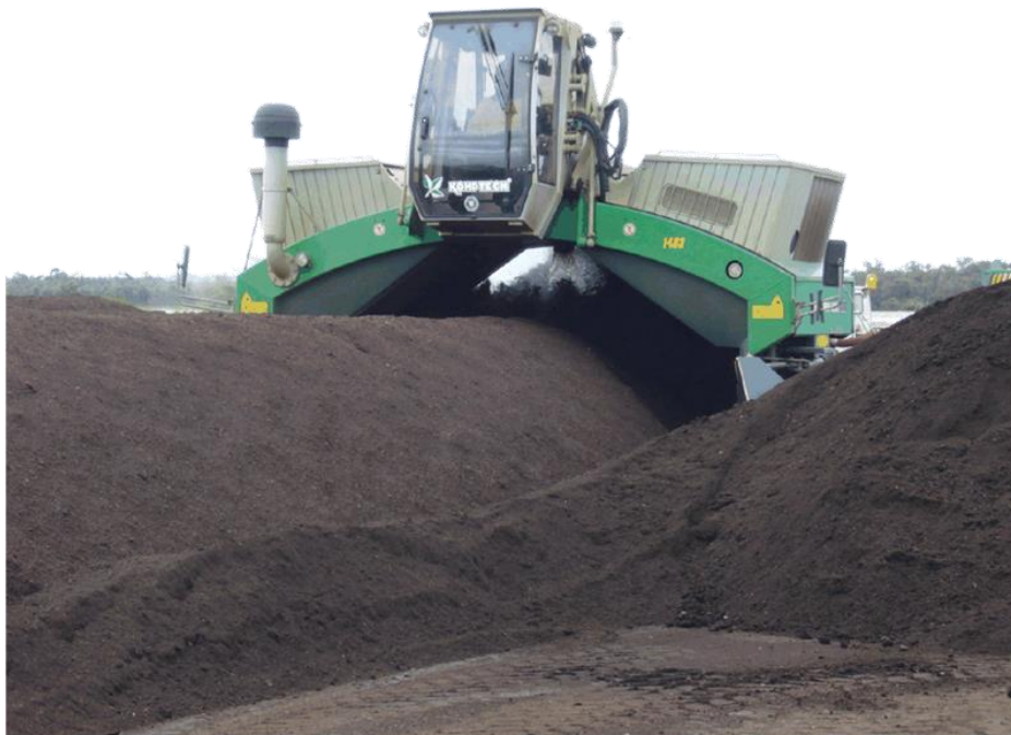
Top over turner that applies water to the windrow during the turning process
